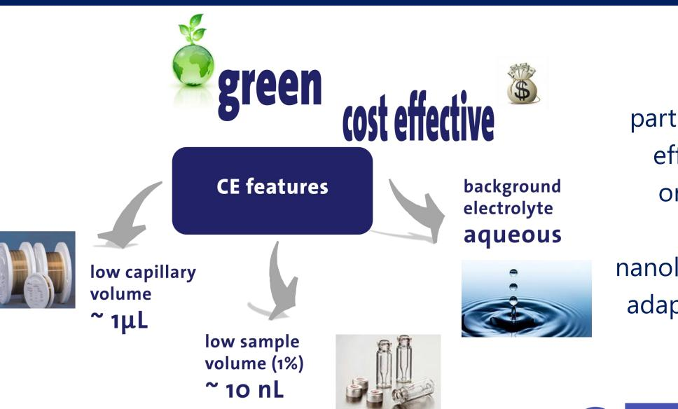
The use of **capillary** electrophoresis (CE) is particularly appropriate for costeffective drug control since no organic solvent is needed and injection volumes are in the nanoliter range, which is perfectly adapted to the low availability of reference substances.
